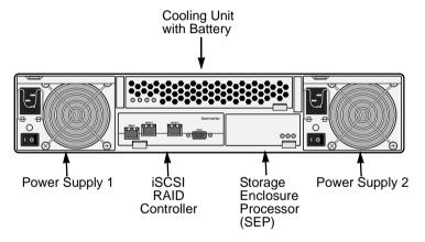
Figure 4. VTrak M300i/M200i Rear View (M300f/M200f and M300p/M200p have different controllers)
